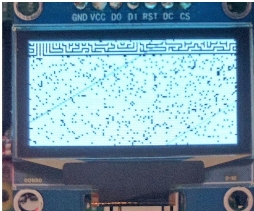
Fig. 1: Display corruption due to using driver for incorrect controller when running the maze.py example
