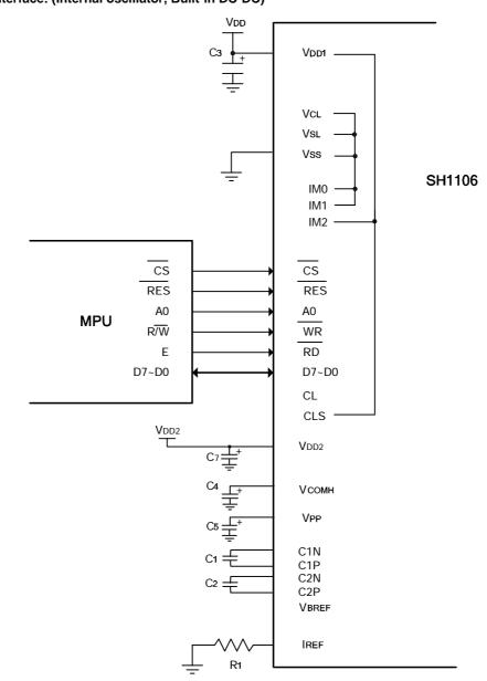
2. 6800 Series Interface: (Internal oscillator, Built-in DC-DC)
