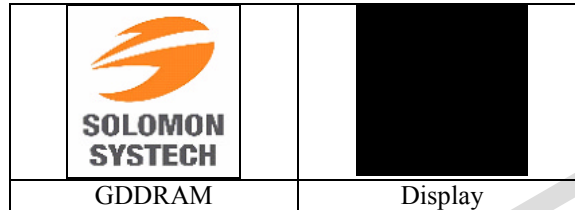
Figure 10-7 : Example of Entire Display OFF
